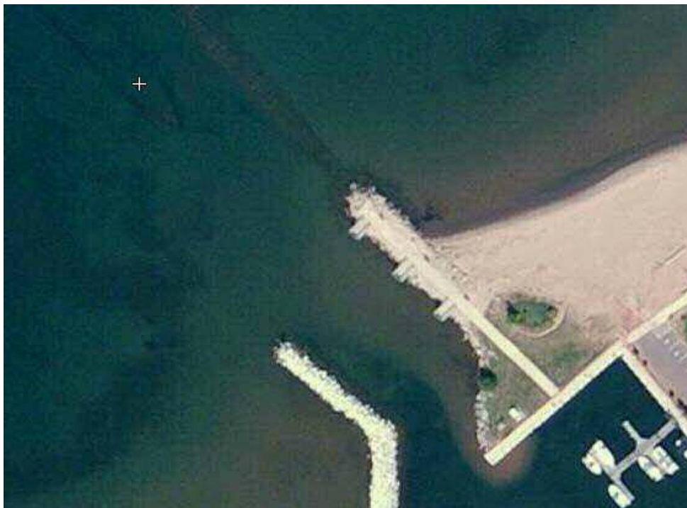
Photo 2: Harbor Entrance prior to 2012 dredging – Photo from Google Earth Note: Sediments in channel & along north pier
