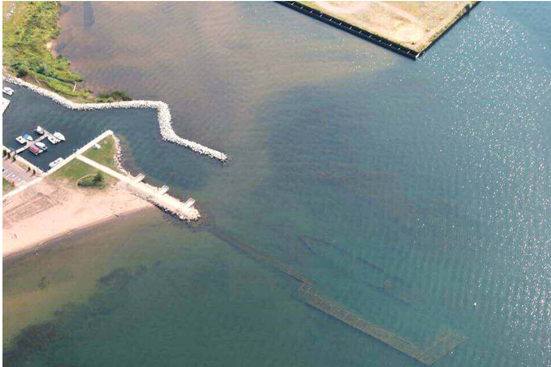
Photo 3: Harbor Entrance in August 2013 – Local photo Courtesy of Derik Dougovito Note: Dredged Channel (2012), Sedimentation from Falls River, Sunken boat “Northerner” and old crib pier
